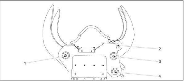
3. Check the tightness of the cutting blade bolts (1-7).
