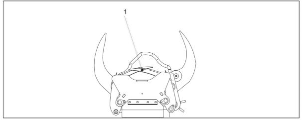
2. Place the tree bundle between the cutting side jaws (1) and the cutting blade (2). The collector unit (3) must be closed.
