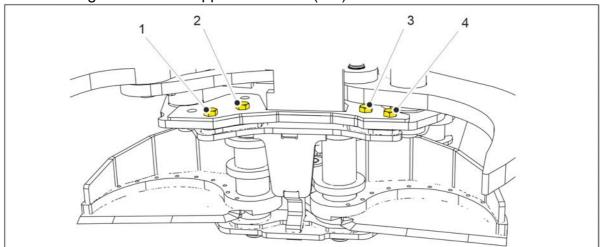
2. Check the tightness of the bottom front bolts (1-2).
