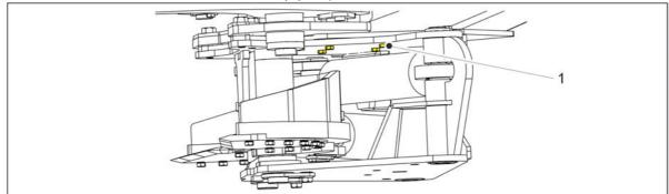
7. Attach the inflow and outflow hydraulic hoses for the guillotine unit.
