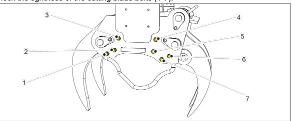
4. Check the tightness of the bottom bolts (1-3).
