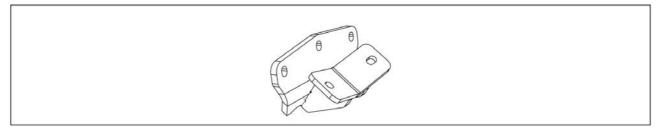
The foot is available for use with the excavator adapter. The foot is used as a support point for moving the excavator at the work site. The foot is attached to the back bottom side of the excavator adapter.
