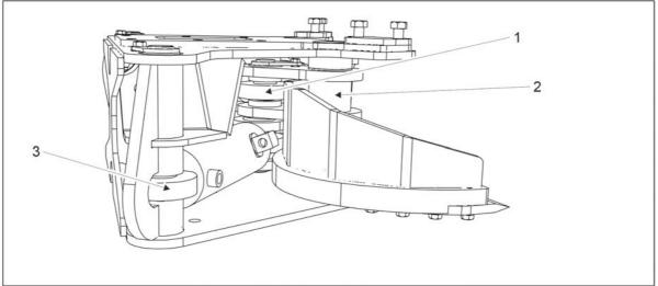
2. Apply grease to the grease nipples on the left side of guillotine unit (1-3).
