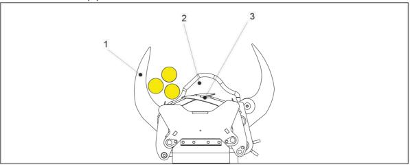
3. To cut the tree bundle, close the jaws (1). Now the jaws hold the tree bundle. The collector unit (2) is closed.
