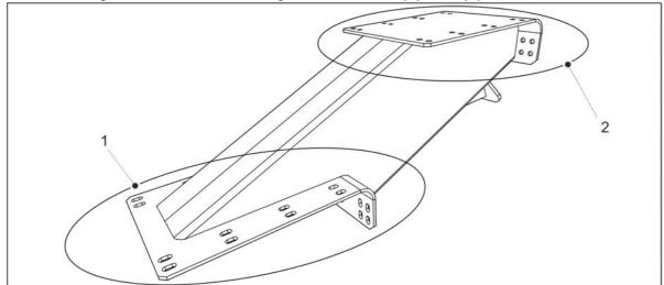
2. Visually check that there are no cracks or fractures on the foot.
